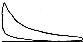
FIG. 34.—Indicator diagram from Bruce-Macbeth engine.
